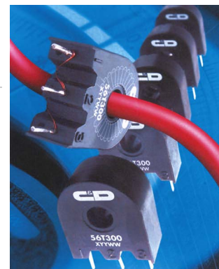
The 5600 current-sensing transformer series offer 500V-dc isolation in 50- to 300-turn versions.
